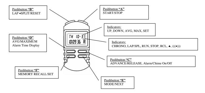
The indicators in this illustration will appear only when a particular mode or function is activated by pressing a pushbutton.
